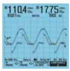
You can use the ScopeMeter 123 to check capacitance of a starting capacitor for a single-phase motor.
