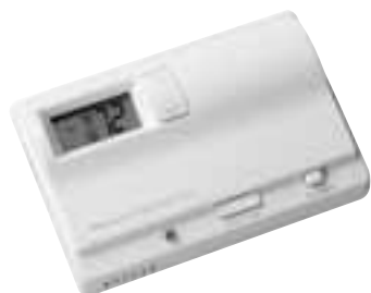
THT02405 (SC3006) 7-Day Programmable, Single Stage Heat / Single Stage Cool or Single Stage Heat Pump, Auto Changeover Terminations: RC, RH, C, W, Y, O, B, G
