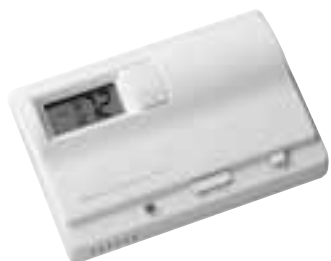
THT02407 (SC3801) 7-Day Programmable, 2 Stage Heat / 2 Stage Cool or 2 Stage Heat Pump, Auto Changeover Terminations: R, C, W 1 /O/B, Y1, W2, Y2, G, S 1, S2
